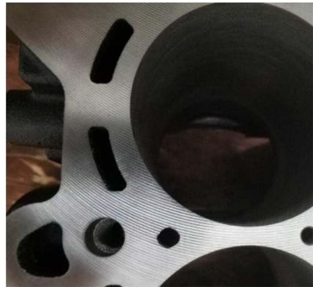
Fig. 27 Partial view of the top surface of engine block after face milling
